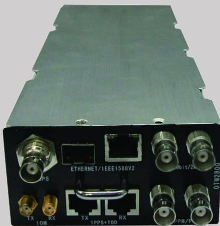
OTM2800 Synchronisation Analyser is specially designed for conducting clock synchronisation of PTN or Packet Ethernet.
