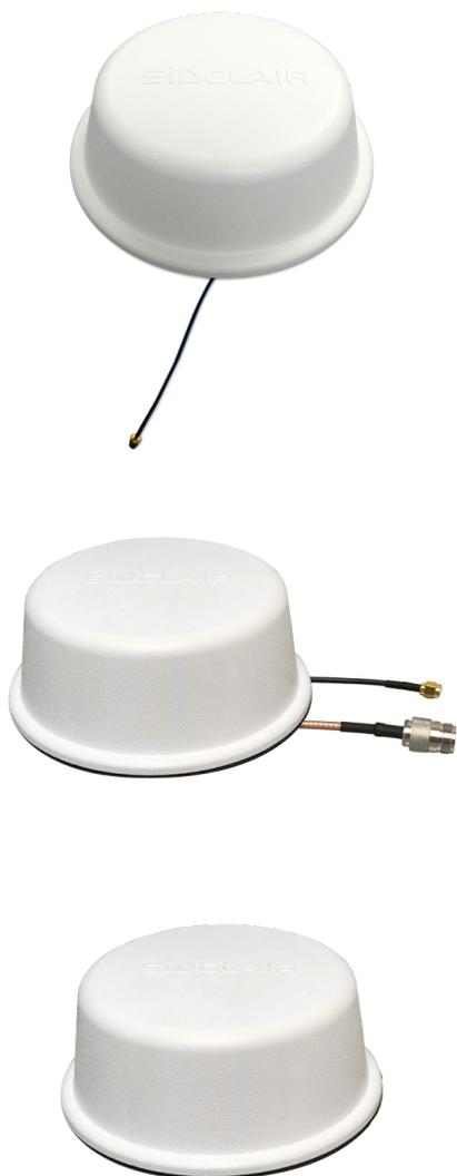
**SM601 Series:** the SM601 series is a 2-in-1 antenna. The RF port covers all the bands for 2G, 2.5G, 3G cellular, LTE 700-2600 MHz. The embedded GNSS antenna utilizes a high-performance LNA that offers outstanding performance. It features a rugged design with UV resistant radome and IP67 rating for reliability and long life in harsh environments. The compact size and low profile allow it to blend easily in any environment and can be mounted on a vehicle rooftop by drilling only one hole.
