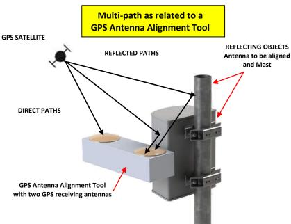
The error caused by multi-path is dependent on the GPS satellite geometry, so that in some cases, the error may be negligible, but in other cases, it can be up to 3° or more. As can be seen from the images above, one of the GPS receiving antennas is receiving a signal from the GPS Satellite that is reflected off the mast and antenna to be aligned. The path of the reflected signal is longer than the direct path, resulting in an azimuth error.
