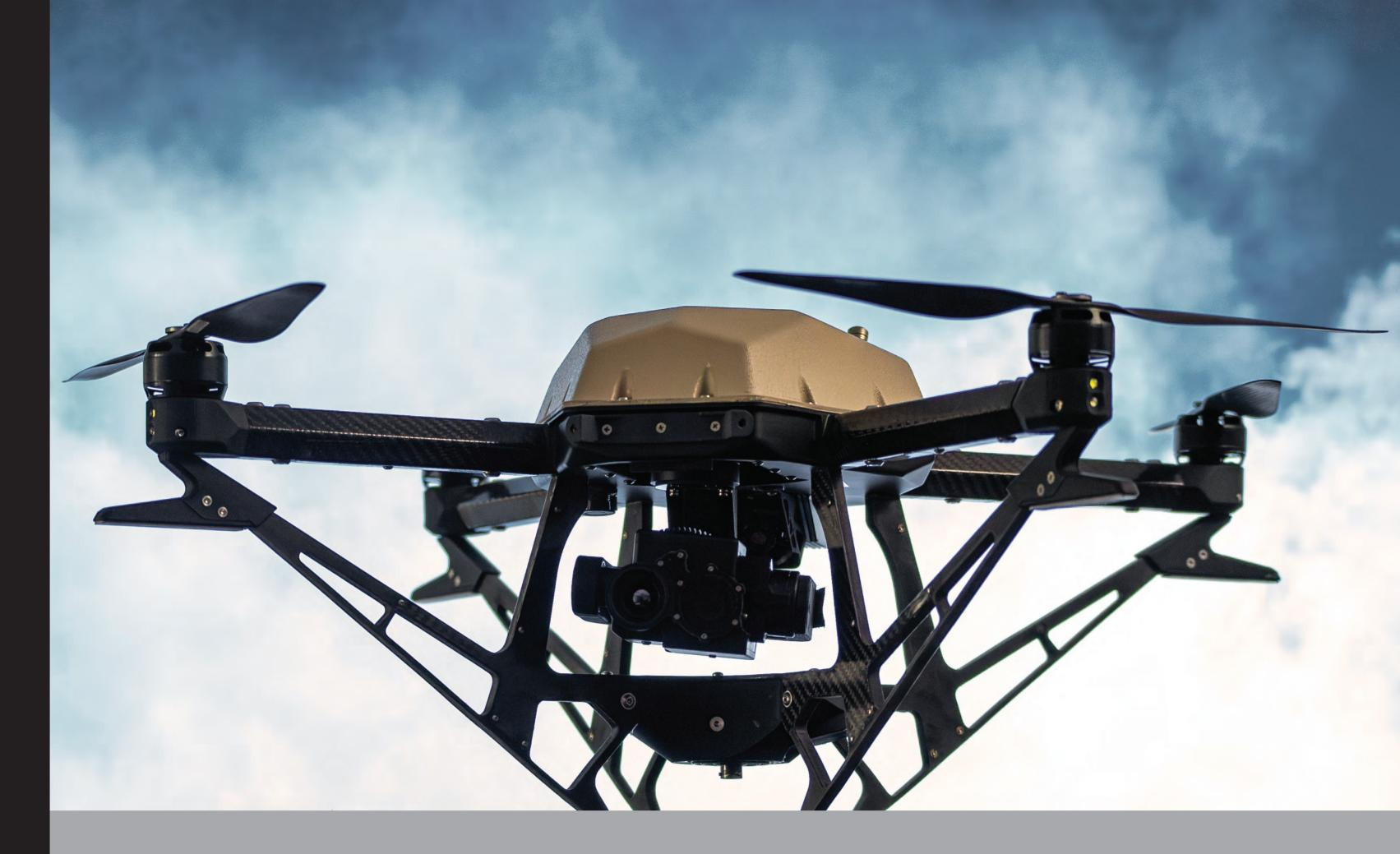
HOVERFLY SENTRY is a VTOL multirotor TeUAS powered from the ground using a highly engineered resilient tether. As a persistent, multi-day, aerial platform it is currently used for ISR and Communications Relay (VHA). With rapid deployment and rapid collapse, it can be mounted on and operated from moving vehicles, on the ground, and on buildings, to enhance and enable new missions. As a VHA, Hoverfly Sentry is the key to reliable communications and survivability while on the move.
