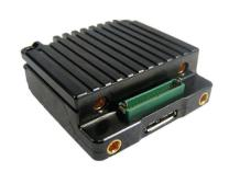
The SOLO8 Software Defined Radio is an COFDM digital video transceiver from Domo Tactical Communications (DTC), designed specifically for Point of View (PoV), UxV, body worn and concealment applications.
