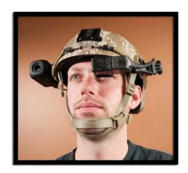
The Liteye HMTI-HMD is a RUGGED, Head Mounted Thermal Imager.
