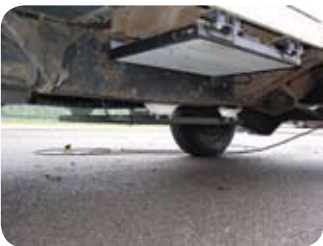
High power planar spiral antenna mounted under vehicle provide countermeasures
