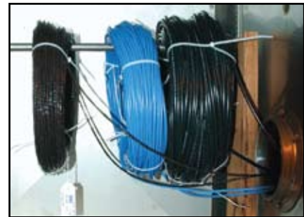
The cables were tested, as suspended, in a high temp oven.
