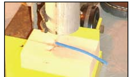
In the cold impact test, after the cable is cooled an aluminum weight smashes against it.
