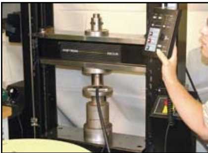
The Instron crushing device.
