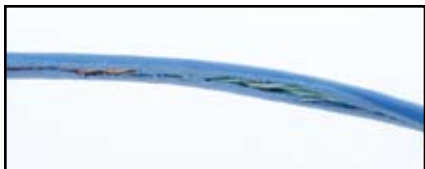
Commercial cable after 25 cycles.
